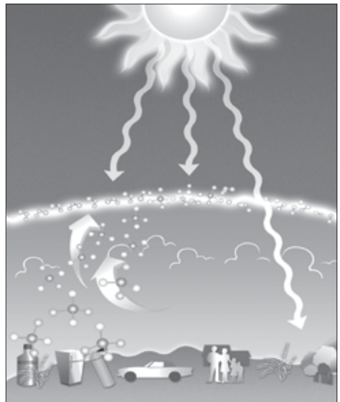
CFCs were used for many different purposes, including refrigerants in mobile A/C systems prior to about 1992. Leaks and other releases allow them to enter the atmosphere.
